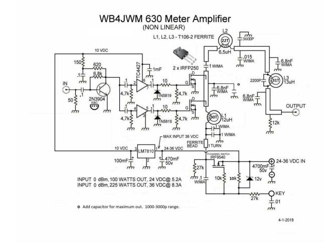
Input 0dbm drive for 200 watts out at 36VDC or 100 watts out at 24VDC.
